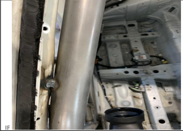
PHOTO 7 FRONT ROLLBAR TO "A" PILLAR ATTACHMENT
