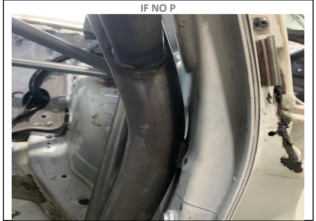
PHOTO 8 MAIN ROLLBAR TO "B" PILLAR ATTACHMENT
