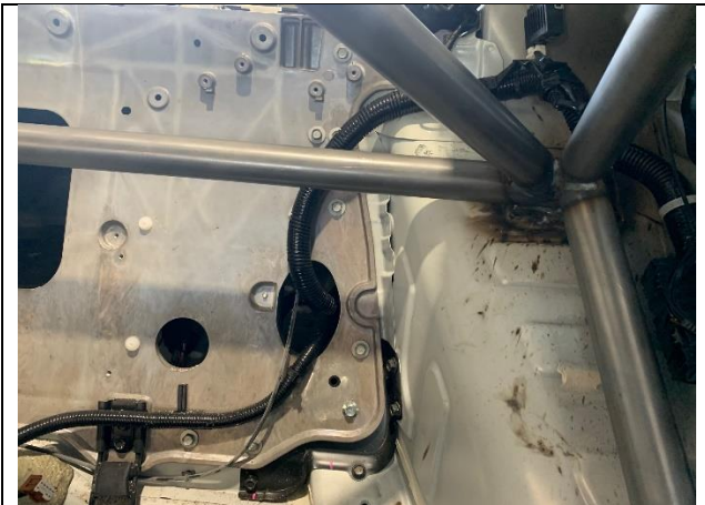
PHOTO 5 REAR BACKSTAY TO BODYSHELL ATTACHMENT
