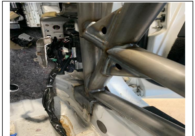
PHOTO 6 FRONT ROLLBAR TO FLOOR ATTACHMENT
